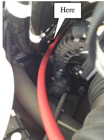
Figure 4: Staged photo of power cable against alternator
