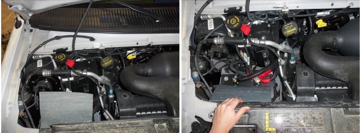
Figure 7: Location of under-hood studs. The left picture shows the studs covered. Under-hood routing will vary.
