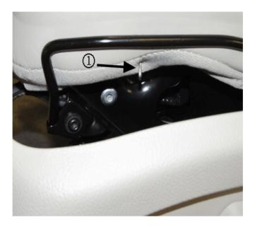
**Note:** Some seats may have a single hog ring (1) at either or both front corners of the seat. For the outboard corner repair, it will be necessary to remove this hog ring to fully release the J-channel from the seat frame. For the inboard corner repair, leave the existing hog ring intact.
