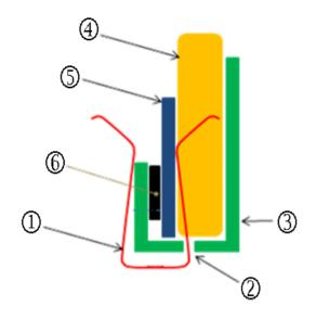
**Note:** A cross section of the clip installation is shown in the illustration above. Ensure the clip (1) is inserted through the slit (2) in the seat material (3), between the foam (4) and the seat frame (5), capturing the material and J-channel (6).
