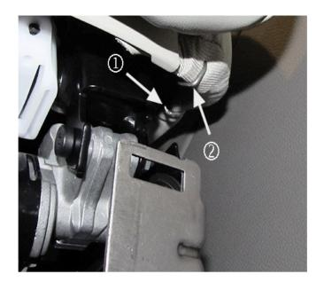
Note: The graphic above shows the original (1) and the added hog ring (2) on the passenger front seat.
