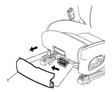
8. Reinstall the front seat adjuster finish cover. Refer to Driver or Passenger Seat Adjuster Finish Cover Replacement in SI.
