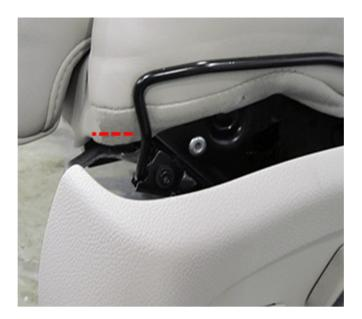
5.1. Fold the J-channel back under the cover fabric material and note the location of the bottom edge of the channel through the material.
