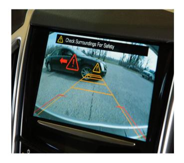
The Rear Cross Traffic Alert (RCTA) System. On vehicles with RCTA, a red warning triangle with an arrow may
