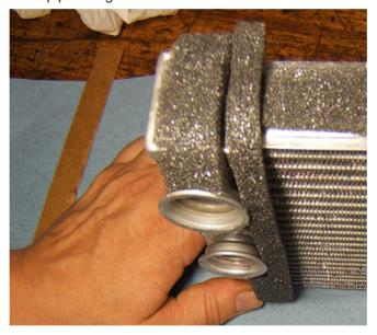
4. Wrap the foam seal around the tank end. Ensure the ends overlap as shown.
