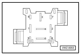
Plug the unplugged starter relay -1- into the empty right-hand relay socket on the additional relay housing.
