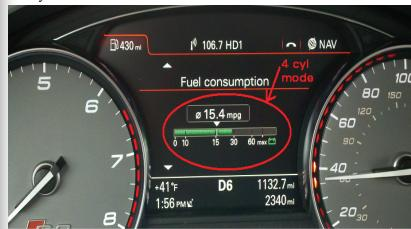
When the engine is in the 4-cylinder mode, cylinders 2, 3, 5, and 8 are deactivated using the Audi Valvelift System (AVS). During this mode, the camshafts are shifted to a round lobe that does not create any valve lift. Fuel injection and ignition are switched off. Engine vibration is reduced by the new motor mounts, and the Active Noice Control (ANC) turns on to minimize any discomfort to the passengers. See SSP 920223 for more information.
