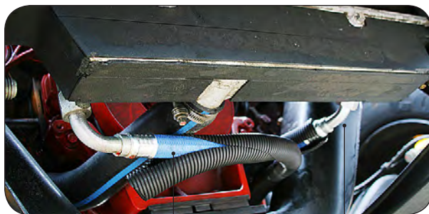
Transmission oil hoses
