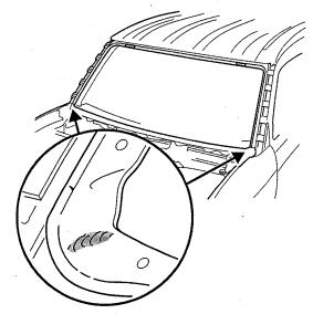
Using a hammer, carefully flatten the high spots so they are even with the rest of the area. If needed, apply touch-up paint to the flattened areas.
