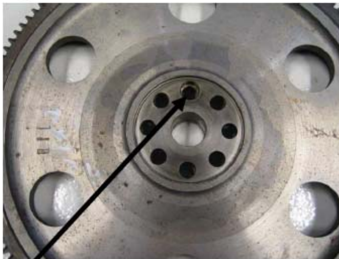
Enlarged hole to fit over collar
