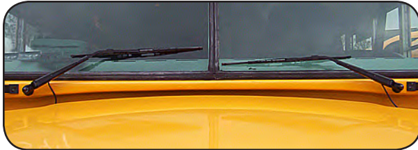
Wipers not properly aligned
