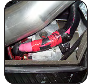
After: Cable secured to prevent contact with CAC tube.
