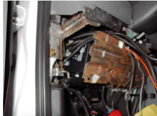
Gateway Module installed on left side of knee bolster bracket in vehicle
