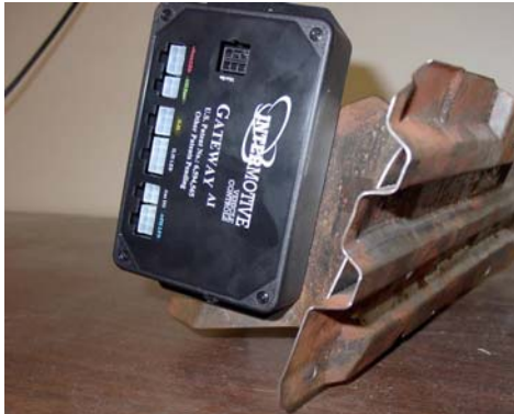
Gateway Module located on left side of driver knee bolster bracket
