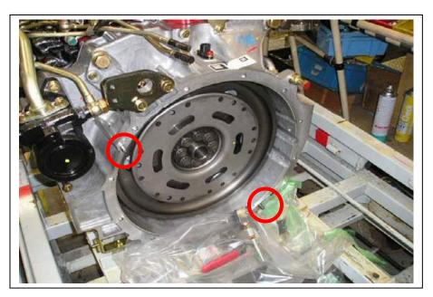
(stock engine) please insure that both dowel pins are present as shown during installation
