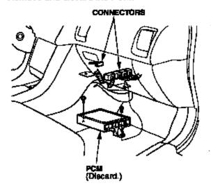
Install the new PCM, and torque the bolts to 12 Nm. (8.7 lb-ft).
