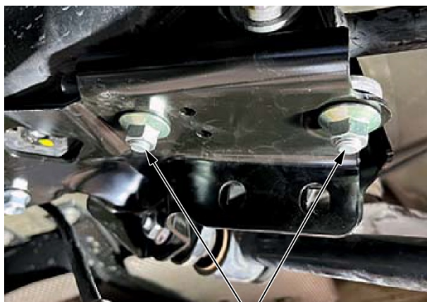
10x30 CARRIAGE BOLTS WITH 10mm FLANGE NUTS
