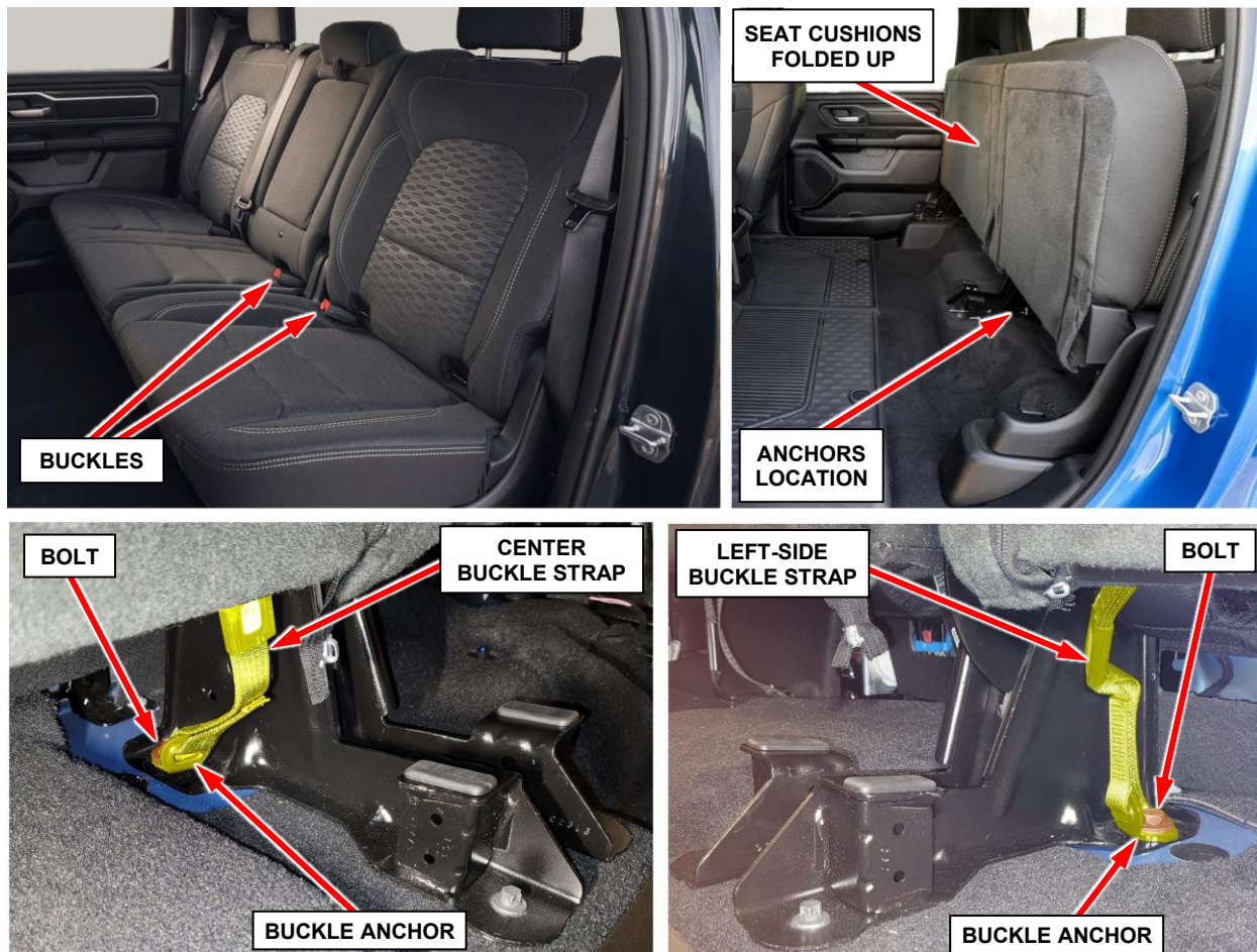
Figure 1 – Second Row: Center and Left-Side Seat Belt Buckle Anchors
