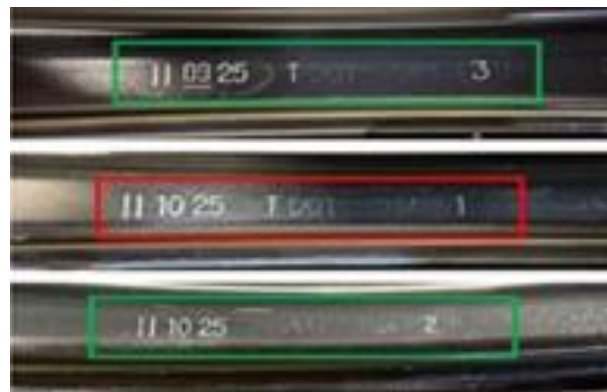
Figure 2 – Three examples: Good Date Codes in Green Boxes, Bad Date Code in Red Box
