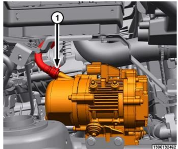
Figure B9 – EHPS Pump Return Hose
