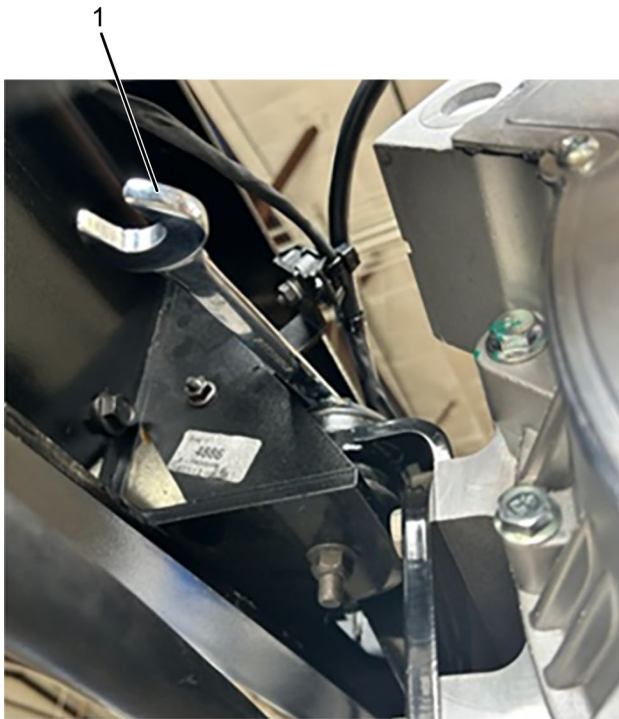
Figure 2. Drive Motor Upper Mounting Bracket Fasteners
