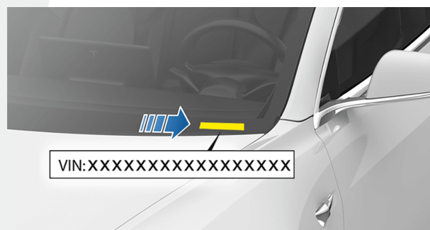
Figure 3 – VIN location on vehicle
