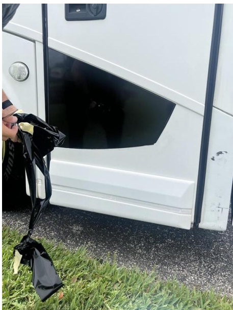
Figure 7: Vinyl Cut, Edges Adhered
