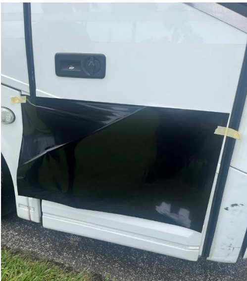
Figure 3: Masking Tape - Holding Vinyl
