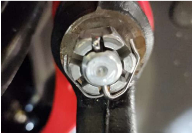
Upper Control Arm Ball Nut & Cotter Pin (Figure A)
