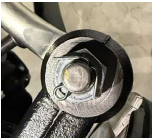
Tie Rod End Nut & Cotter Pin (Figure B)
