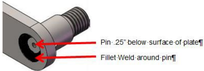
Fillet weld around recessed pin
