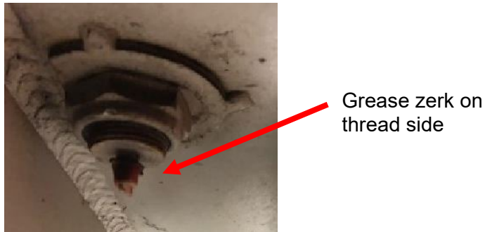
Grease zerk on thread side
