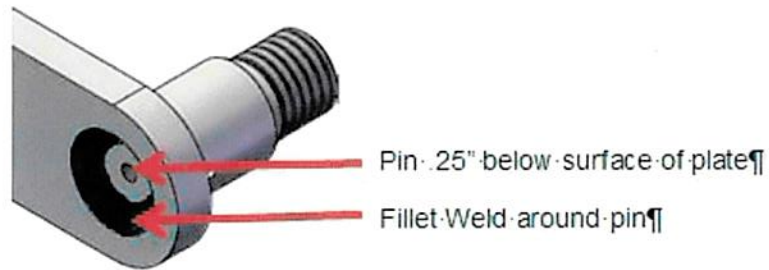
Fillet weld around recessed pin
