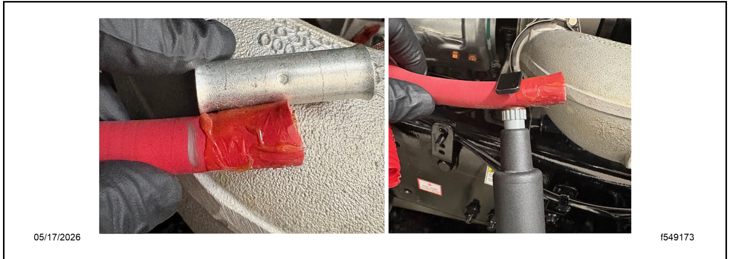
Fig 37, Removing the Insulation
