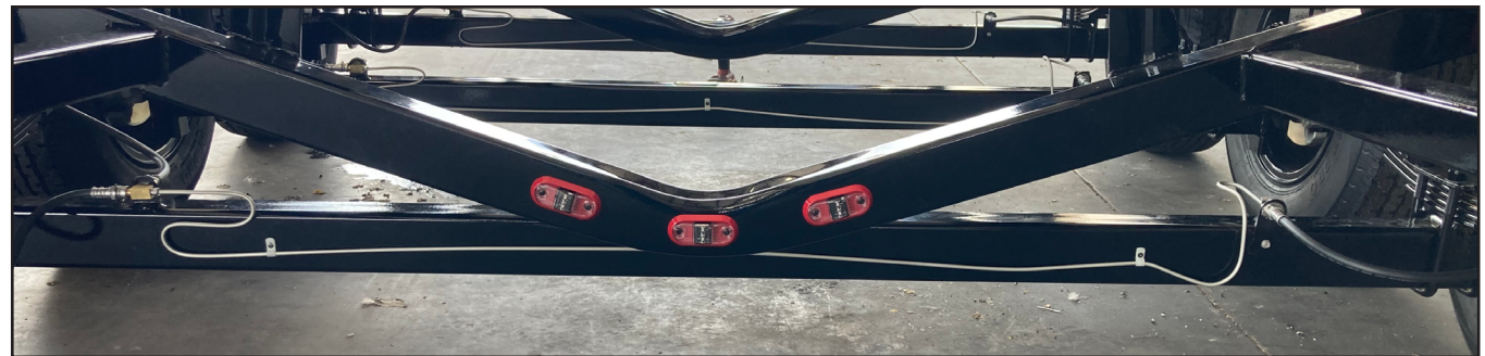
Updated trailer brake line configuration.
