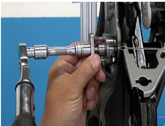
Hold tool flush to bracket.
