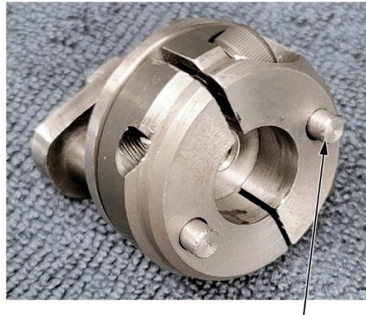
LOADING PINS Protruding, no good.
