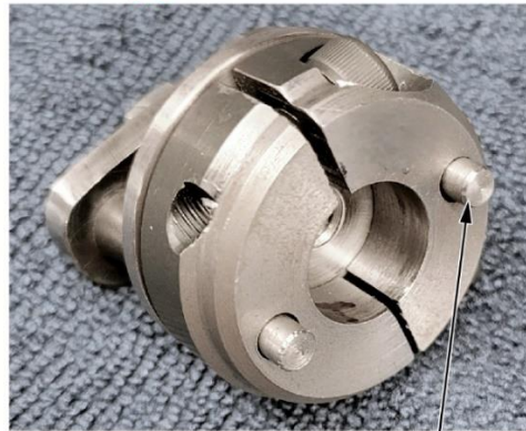
LOADING PINS Protruding, no good.
