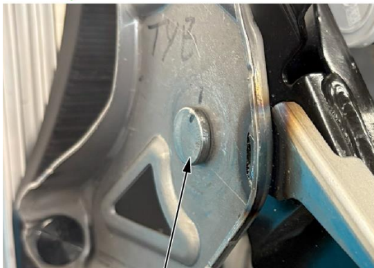
PIVOT PIN Pin is flush. No repair is needed.
