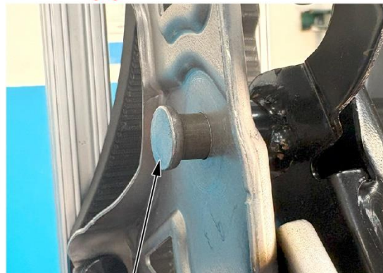
PIVOT PIN Pin is pulled away, not flush. Repair is needed.
