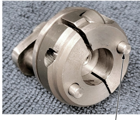
LOADING PINS Protruding, no good.
