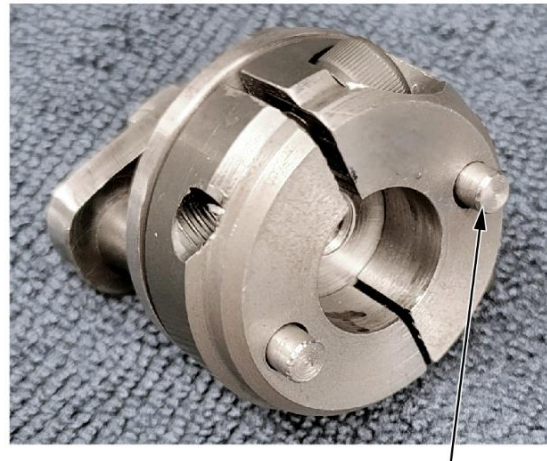
LOADING PINS Protruding, no good.
