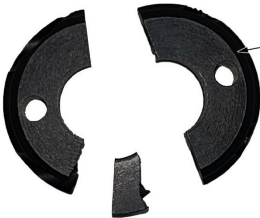
INSPECTION TOOL Broken due to power tool use.
