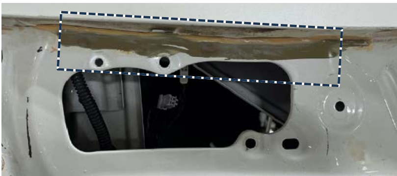
Example of finished sealer removal:
