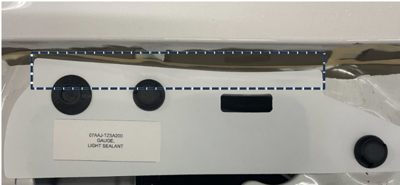
Example of finished sealer removal:
