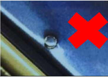
Example: Body panel damage due to a tap being run too deep
