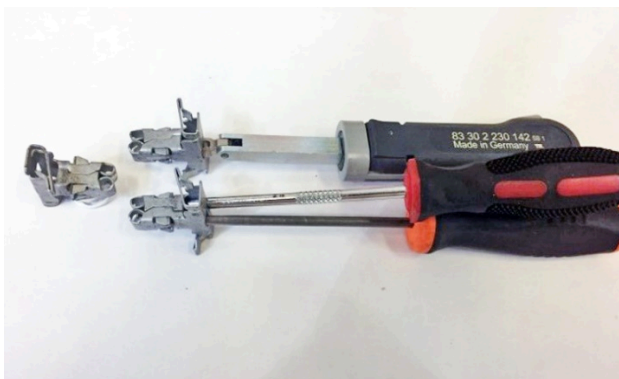
Clip with tool 2 230 142 inserted with spring clips pulled inward by tool
