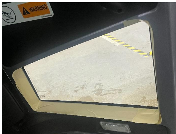
Figure 2: Panels Installed on Inside Lower Glass Window
