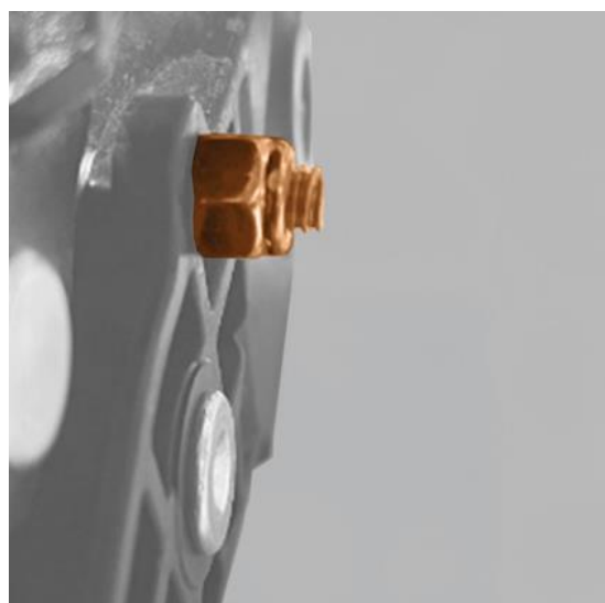
Figure 5 – An Over Torqued Fastener
