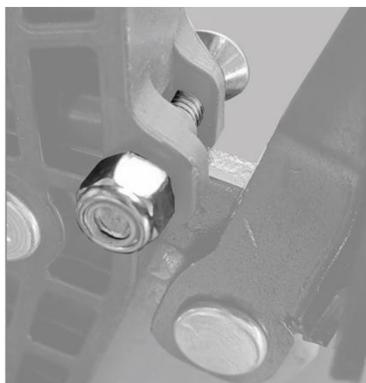
Figure 6 – An Under Torqued Fastener
