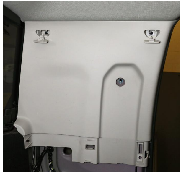
Figure 30 – C-Pillar Upper Trim Panel Fasteners
