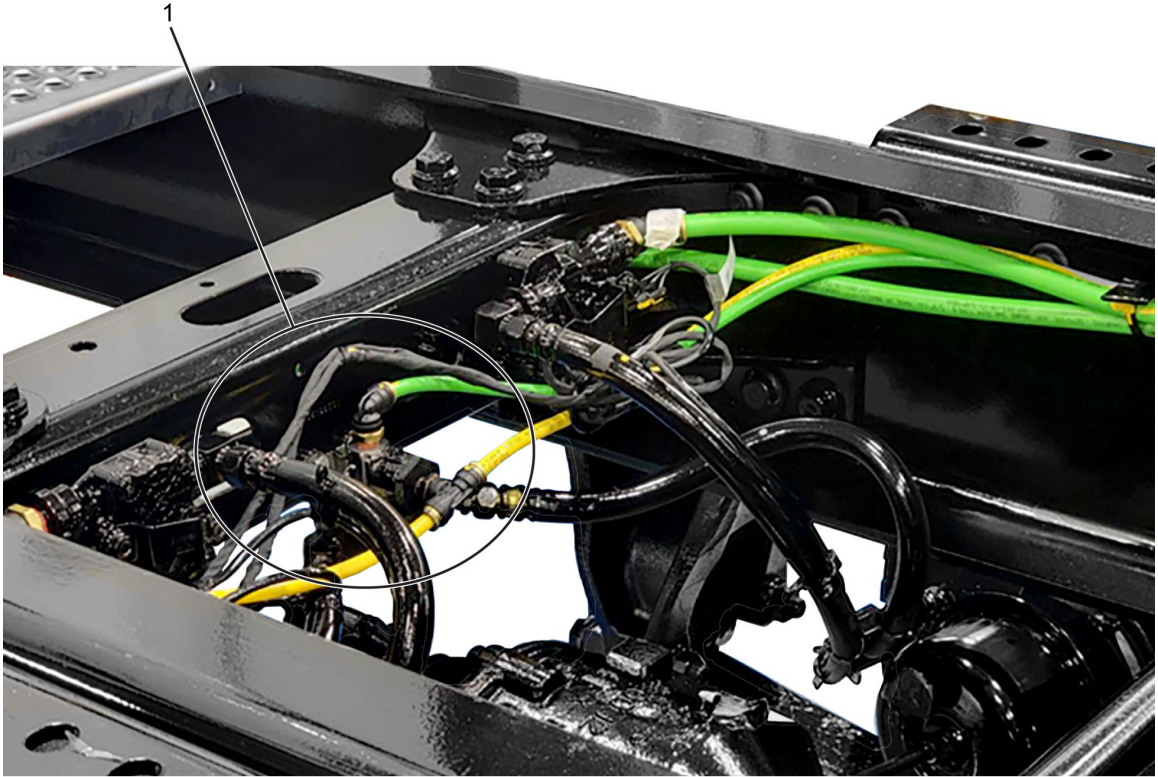
Figure 2. Forward-Rear QR-1C Valve 1. Forward-rear QR-1C valve assembly
