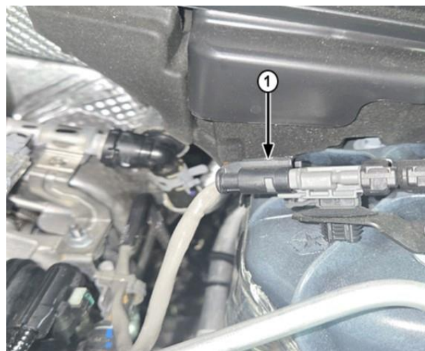
1 - O2 Sensor Wire Harness Connector
