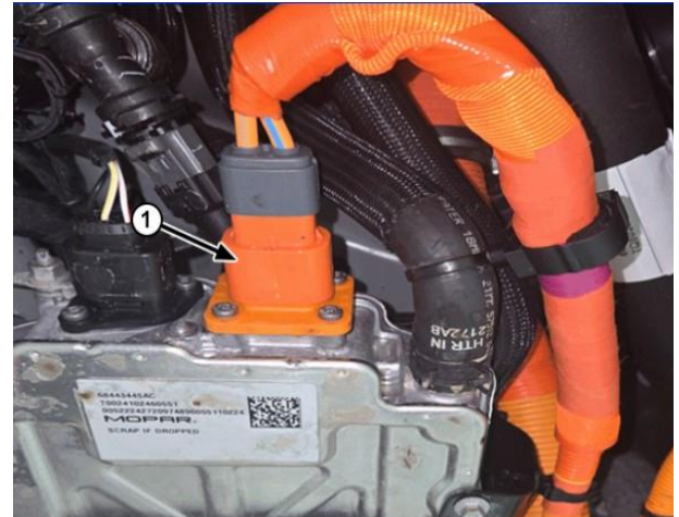
1 - High Voltage Cabin Heater Cable Wire Harness Connector
