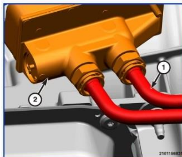
1 - Transmission Oil Cooler Lines 2 - Transmission Heat Exchanger
