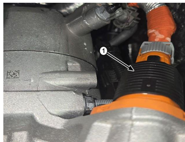
1 - A/C Compressor High Voltage Wire Harness Connector
