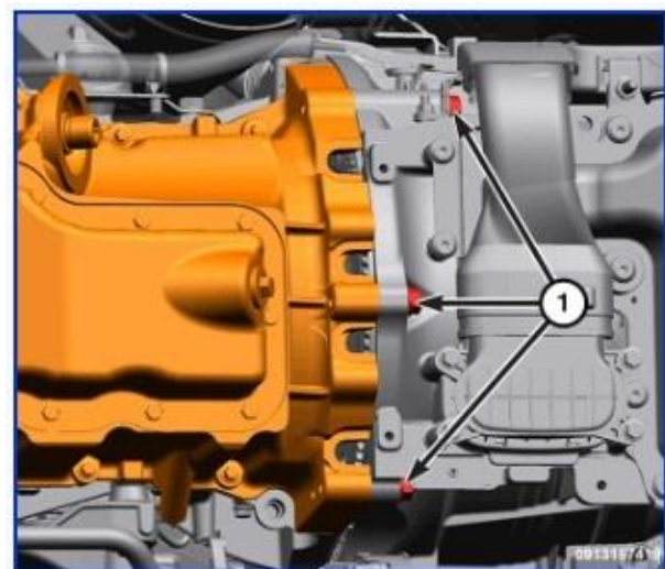
1 - Transmission To Oil Pan Bolts
