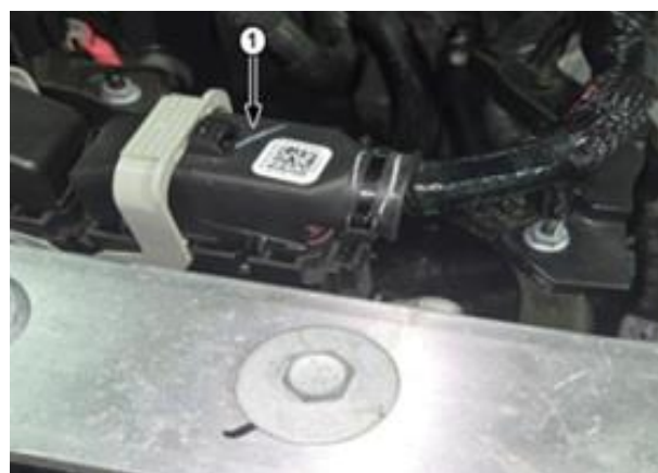
1 - PCM Wire Harness Connector
