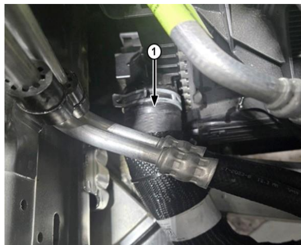
Figure 50 – Lower Radiator Hose
