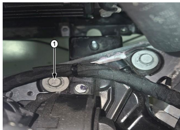
1 - Auxiliary Coolant Pump Bolts
