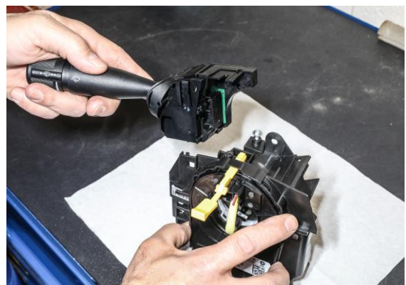
Figure 16 – SCCM Removal and Installation
