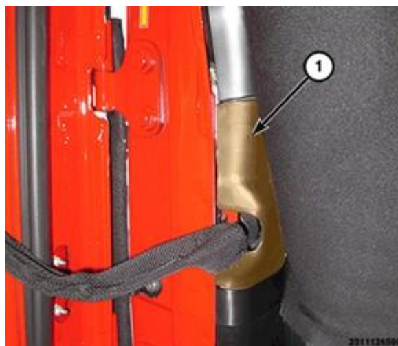
Figure 13 – B-pillar Trim Cover
