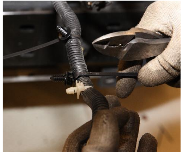
Figure 19 – Wire Harness Retainers
