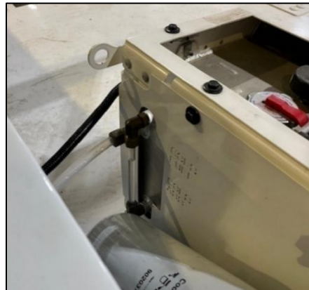
Figure 41: BTMS Sight Glass
