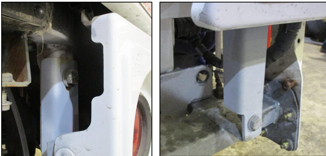
Figure 6a & 6b: Pillar Structure Attachment Points
