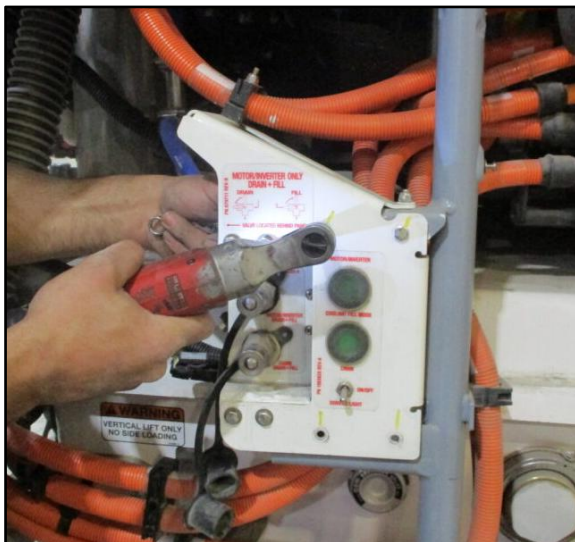
Figure 8a & 8b: Motor/Inverter Coolant Fill Panel
