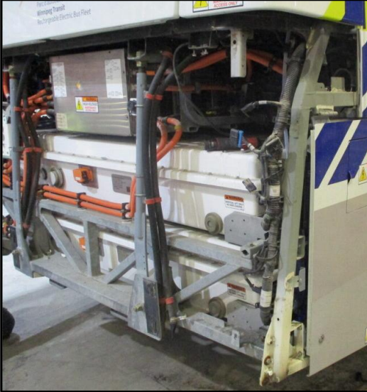
Figure 7a & 7b: Rear Struts, HVAC Drains & HV Cable Mounts
