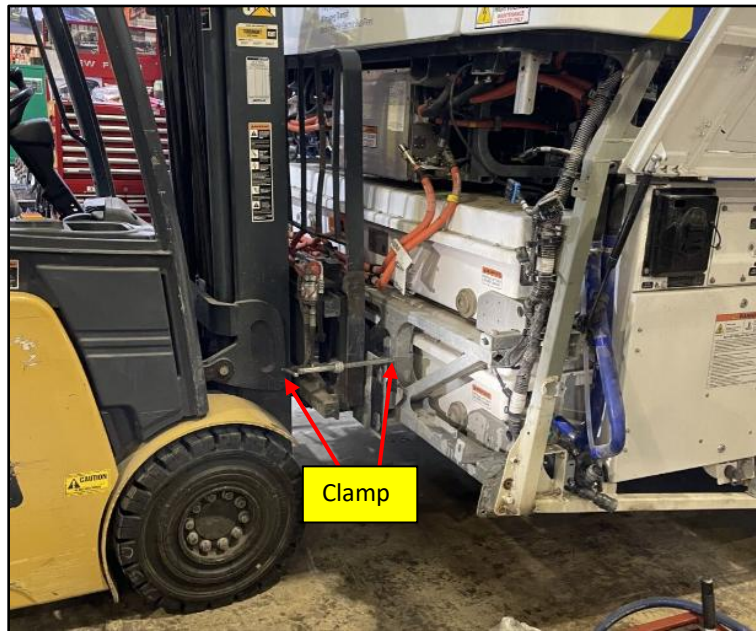
Figure 18: ESS Cradle Secured to Forklift
