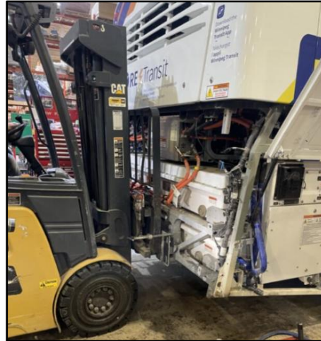
Figure 79: Rear Rack Assembly with ABS Packs Installation
