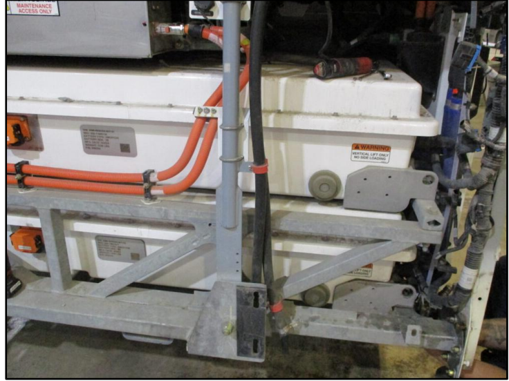
Figure 7a & 7b: Rear Struts, HVAC Drains & HV Cable Mounts
