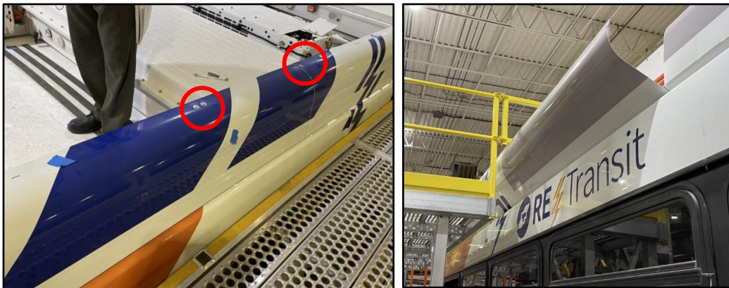
Figure 25: Sidescreen Access Panels
