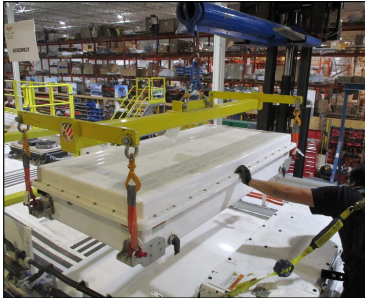
Figure 36: Lifting the ESS from Rooftop
