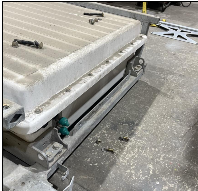
Figure 22a & 22b: Upper Rear Rack Removal
